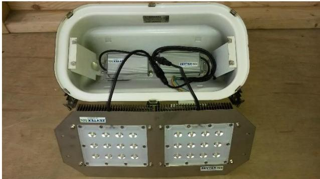
Connect the modules through the waterproof plugs with the drivers.
